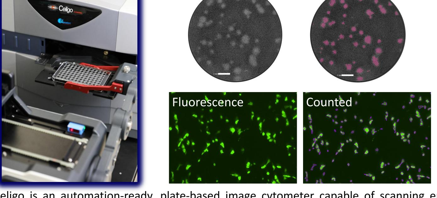
Celigo is an automation-ready, plate-based image cytometer capable of scanning entire wells in bright-field and 4 fluorescence channels in high-throughput. Images are automatically analyzed by Celigo Virology Module to quantify count, size, morphology, and fluorescent intensity. Reports are generated for cell proliferation, fluorescence expression, cytotoxicity, foci counting for viral titer and antibody neutralization assays.
