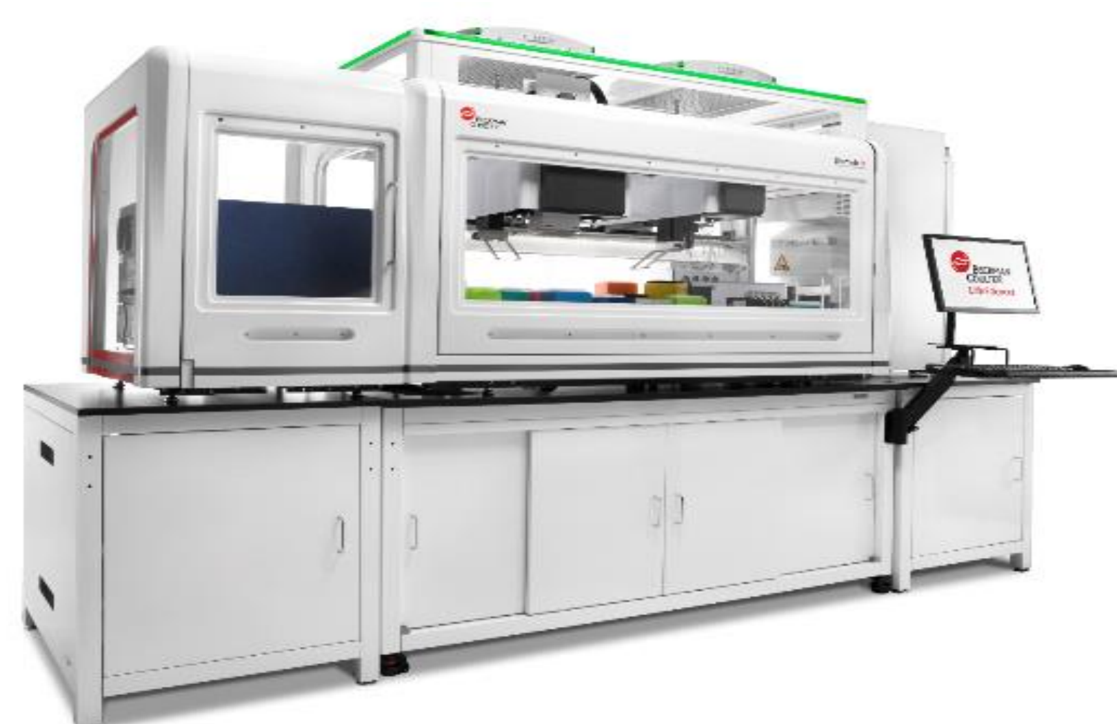
Figure 2. The Biomek i7 Workstation, along with various integrated devices, was used to automate a cell line development workflow.
