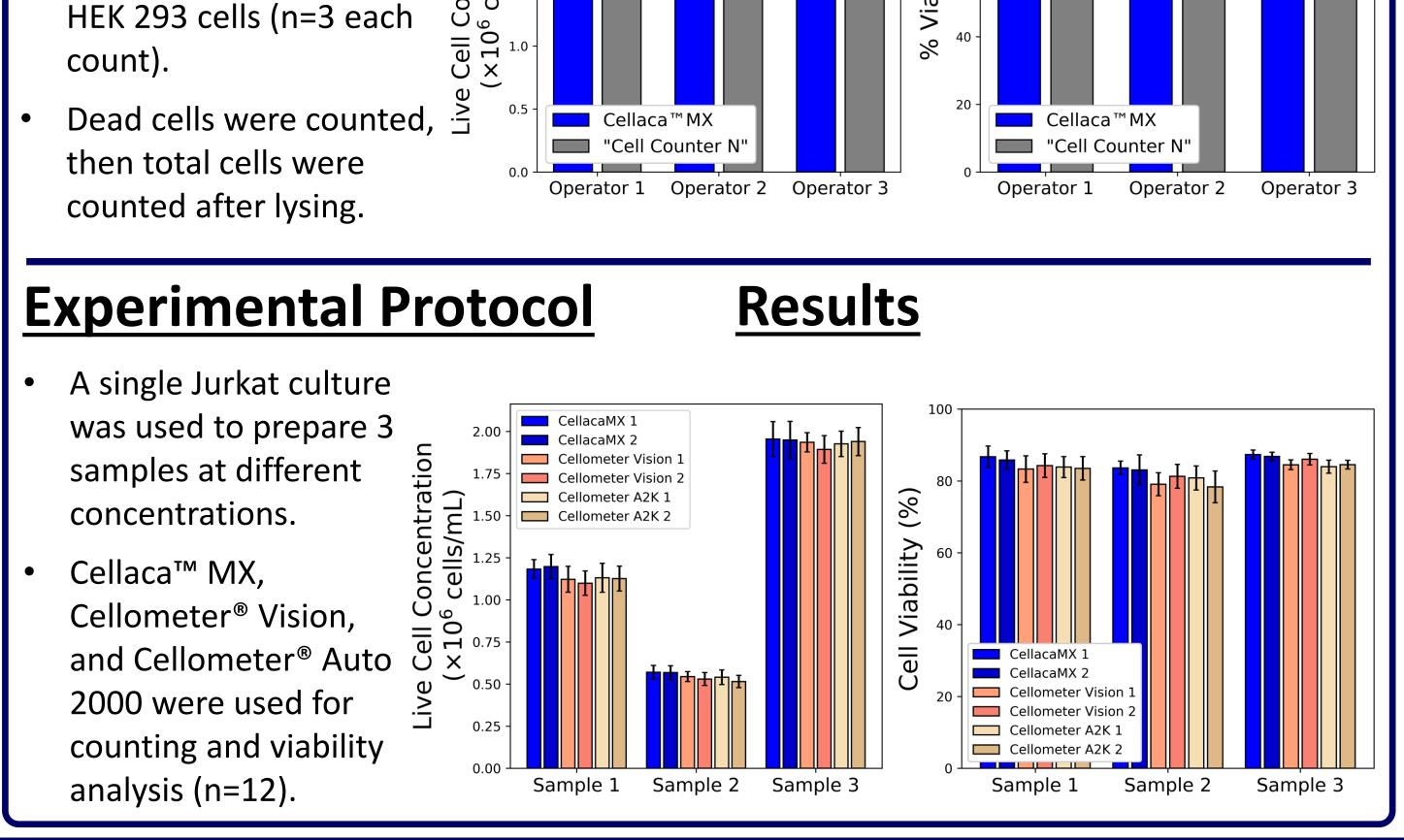
Cell counts by Cellaca™ MX showed high linearity well beyond the instrument's recommended concentration range.
